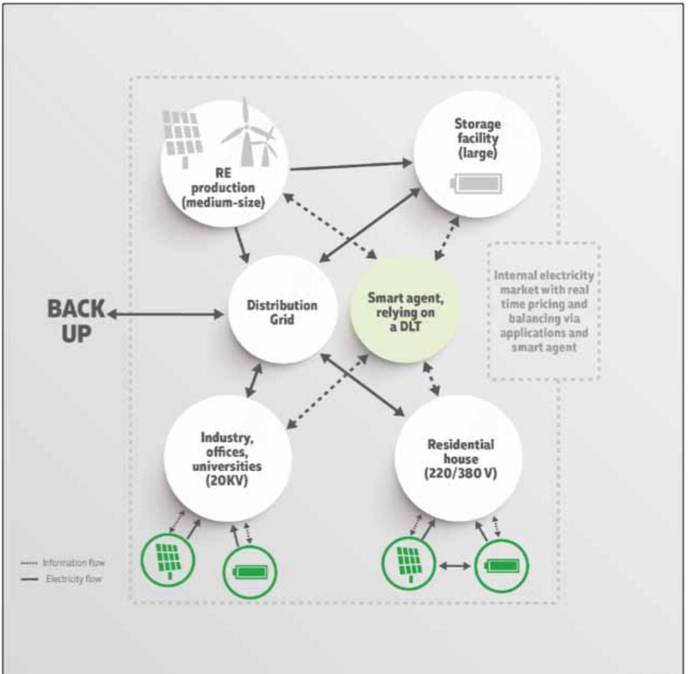
Figure 5: Smart monitoring of a micro-grid
