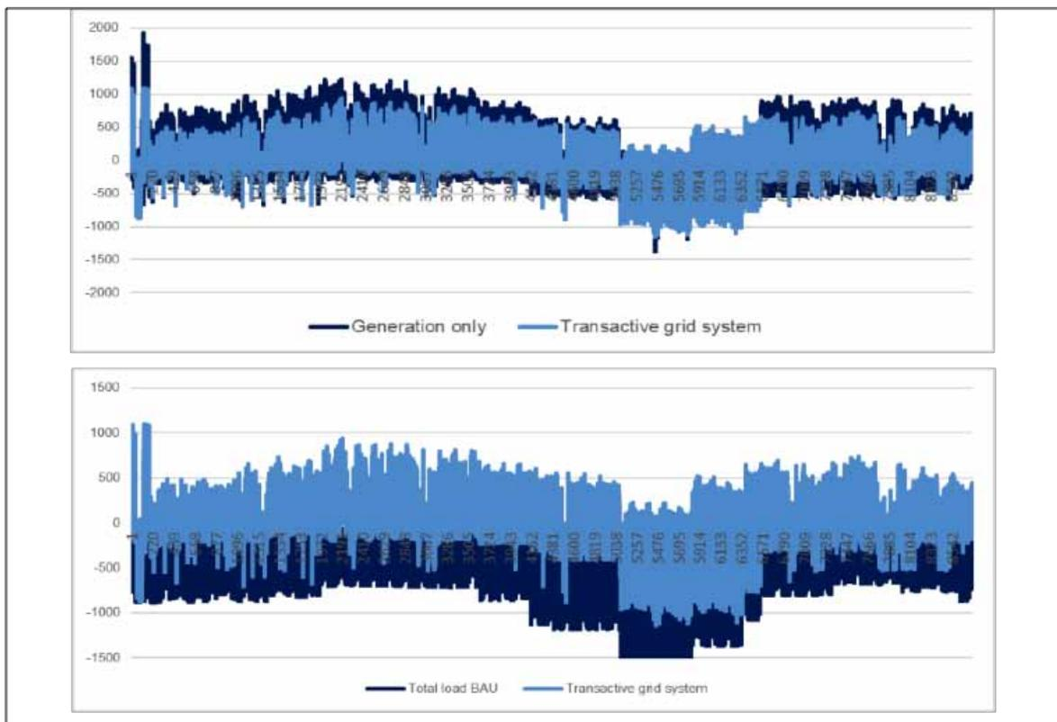
Figure 9: Peak loads reduction and control compared to Regular PV system and Business as Usual - kWh
