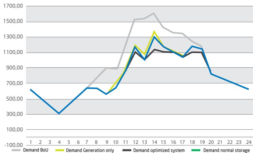
Figure 7: Maximum demand loads comparison - kWh
