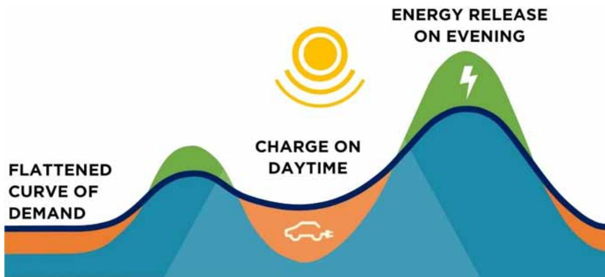
Figure 12: Load shaving with the Vehicles to Grid
