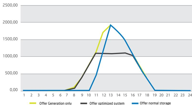
Figure 8: Maximum offer loads comparison - kWh
